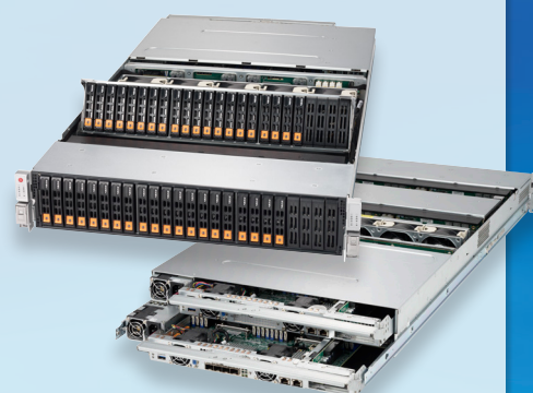
2U 40 Bay Dual Node Server with Dual Port All-Flash NVMe
