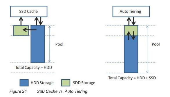
Total storage capacity in auto tiering is a sum of all individual tier capacities whereas in cache, the cache capacity does not add to the overall slower storage capacity. This is one of the key differences. In addition, SSD cache affects rapider than auto tiering because auto tiering will be affected by relocation the data in a period of time. So SSD cache warm-up timeframe is usually minutes/hours whereas tiering warm-up is usually days.
