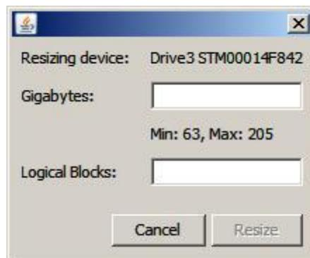
3. Type a value in either the **Gigabytes** text box or the **Logical Blocks** text box. Make sure to enter the value without any commas (,). The system does not recognize non-numerical values.
