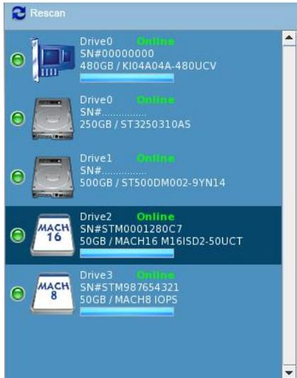
The Devices window lists all the HDDs and SSDs installed in the system. To manage a device, click its icon in the list.
