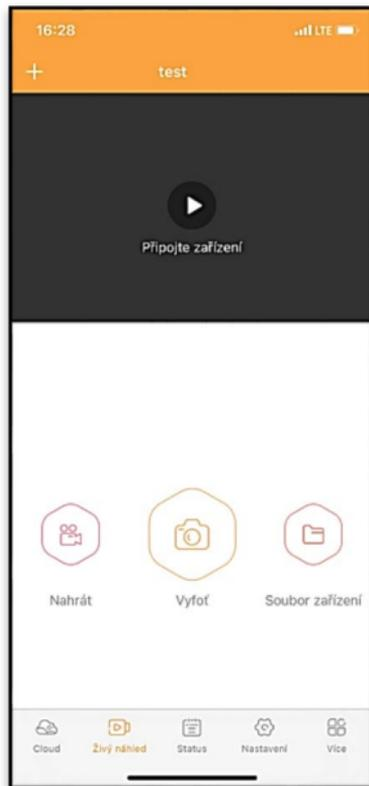
**Recording** - Pressing the "**Record**" or "**Take Photo**" button will capture a photo or video. The action is performed with a delay of a few seconds.
